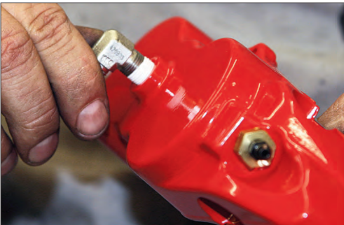
Sequence 21: Remove the protective sticker from the caliper fluid inlet. Coat the inlet fitting with Teflon tape and screw into the caliper with the 90° angle perpendicular to the length of the caliper.
