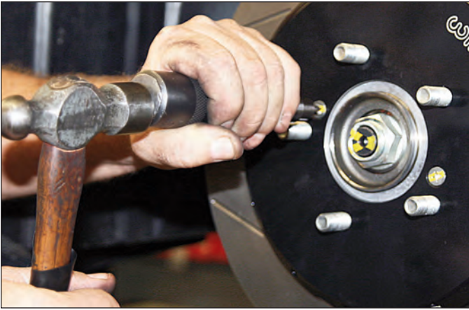
Sequence 19: Reinstall the hat locator screws using an impact screw driver to keep the hat/rotor in place while continuing with the rest of the installation.
