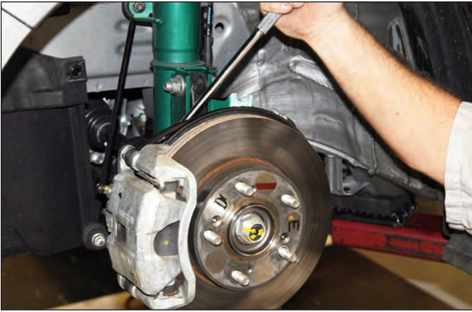
Sequence 7: Using a breaker bar and socket, break loose the caliper mounting bolts from the back side.
