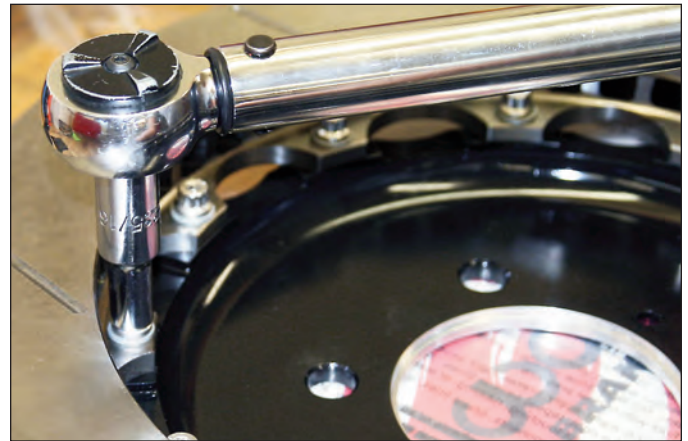
Sequence 17: Place one flat washer over each hole on the rotor mounting tabs. Coat the mounting bolts with red Loctite® 271 and slide through the washer and thread into the hat. Using an alternating sequence, torque bolts to 155 in-lbs.
