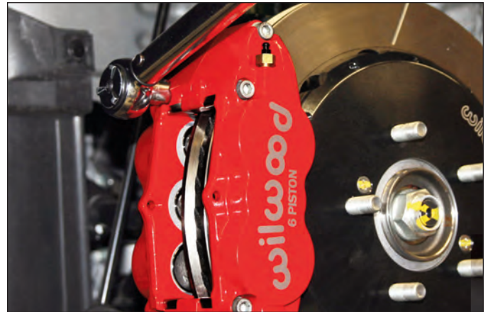
Sequence 23: Secure the caliper with washer and locknut, temporarily tighten. View the rotor through the top opening of the caliper. The rotor should be centered in the caliper. If not, adjust by adding or subtracting shims between the bracket and the mounting ears. Once the caliper alignment is correct, remove the bracket bolts one at a time and apply red Loctite ® 271 to the threads and torque to 65 ft-lb.
