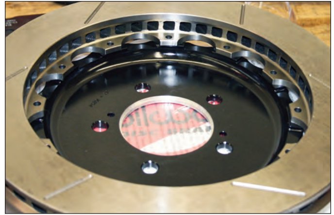
Sequence 16: The hat needs to be bolted to the rotor. Orient the rotor over the hat in the configuration shown above.
